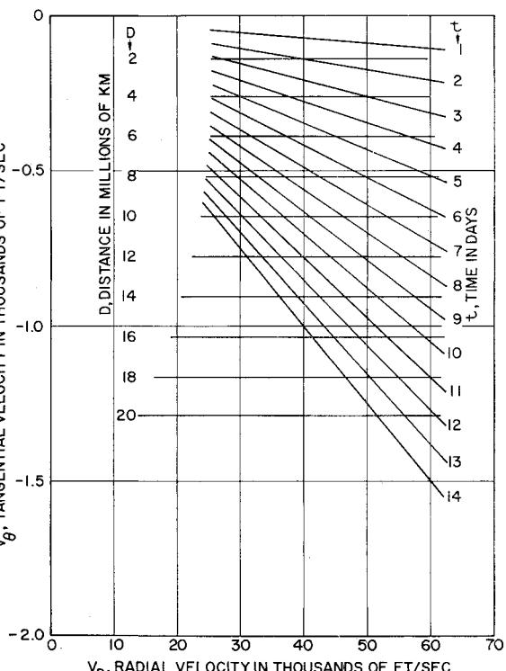
Fig. 3 Satellite tangential velocity vs radial velocity for solar alignment (at given time and distance)
