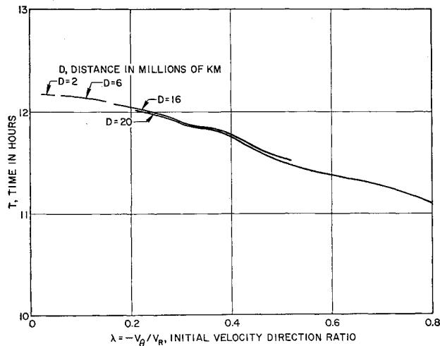
Fig. 6 Satellite solar transit time vs initial velocity direction ratio for solar alignment
