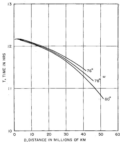
Fig. 7 Satellite solar transit time vs solar alignment distance
