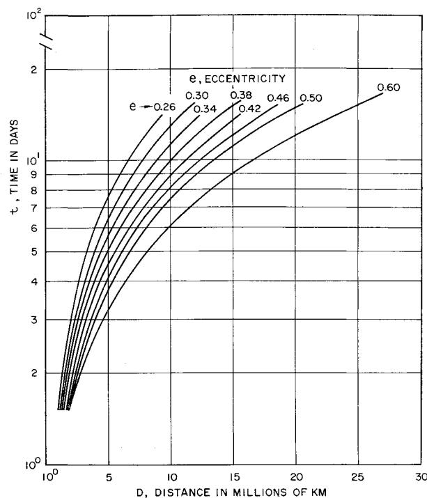
Fig. 2 Time vs satellite radial distance for solar alignment
