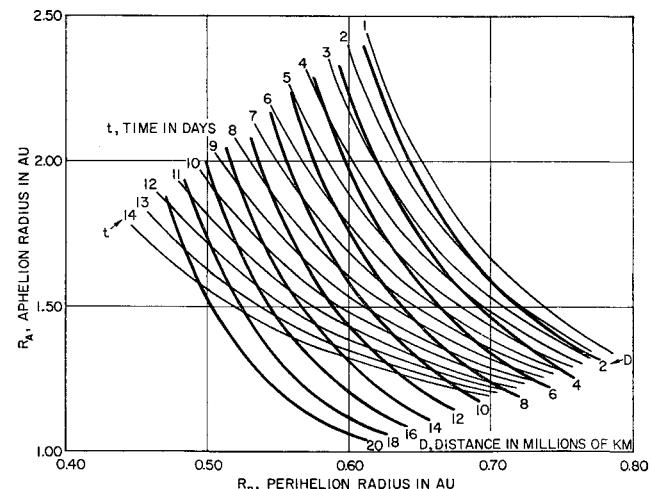
Fig. 4 Satellite aphelion radius vs perihelion radius for solar alignment (at given time and distance)
